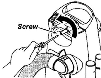
Slide the handle into the opening at the top of the vacuum cleaner.
